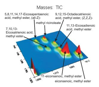
Figure 2: A 3D surface plot of the area indicated by the orange-dashed box in Figure 1. Identifications of select peaks are included.
