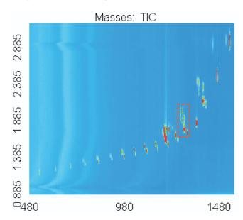
Figure 1: A contour plot of FAME sample #1. The X-axis is retention time on the primary column. The Y-axis is retention time on the secondary column.
